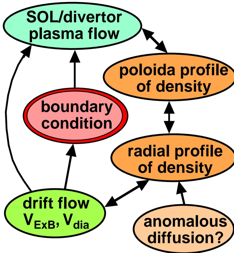
Boundary condition is the key for the 2D structure formation
