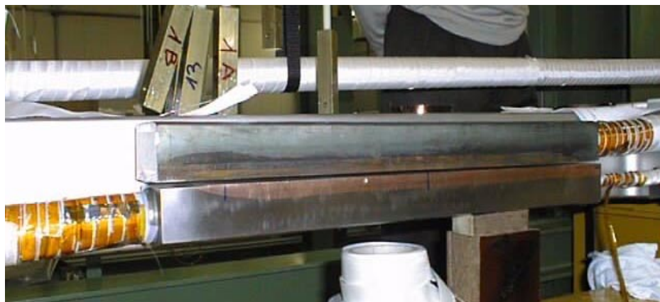
Fig. 5b: Two adjacent terminations of a DP module inner joint before being soldered and clamped together
