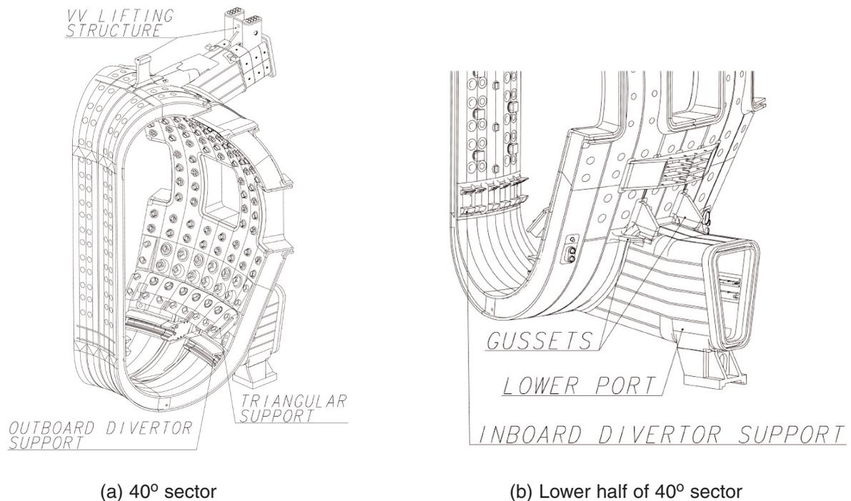
Fig. 1. The ITER Vacuum Vessel
