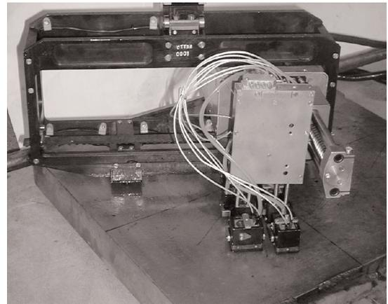
(c) UT inspection system during testing (RFTP)
