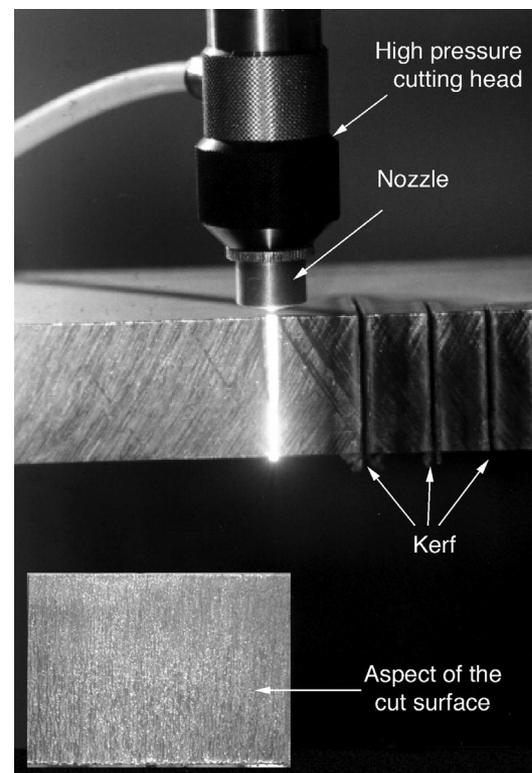
Fig. 8. Thick plate cutting with NdYAG Laser (EUPT) (40 mm thick plate cutting in the photo and 60 mm thick steel, 6 kW NdYAG with nitrogen gas cutting speed: 0.003 m/min)
