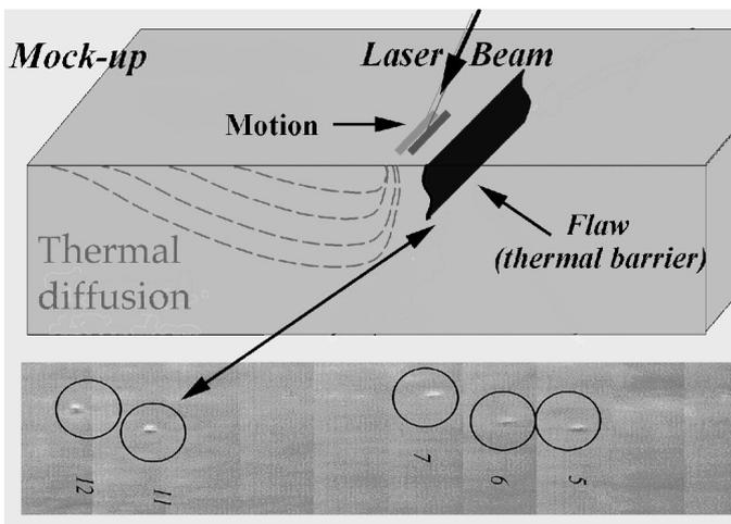
Fig. 7. Photothermal camera as a surface crack inspection method and detected defects in a mock-up test (EUPT)
