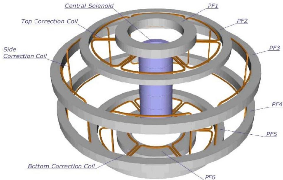
**Figure 4.1-3 ITER Poloidal Field Coils and Error Field Correction Coils**
