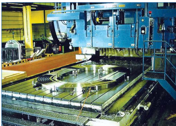
Superconducting Winding of the Toroidal Field Model Coil during fabrication
