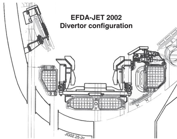
The studies started in campaigns C1-C4 will be further extended this year in all three regimes. The removal of the septum in the divertor (fig. left) will allow an assessment of its contribution in establishing the excellent results of the 2000-2001 campaigns. The final aim is to obtain an integrated operational scenario combining the necessary conditions for use on ITER : high confinement, high density and an acceptable power and particle exhaust.
