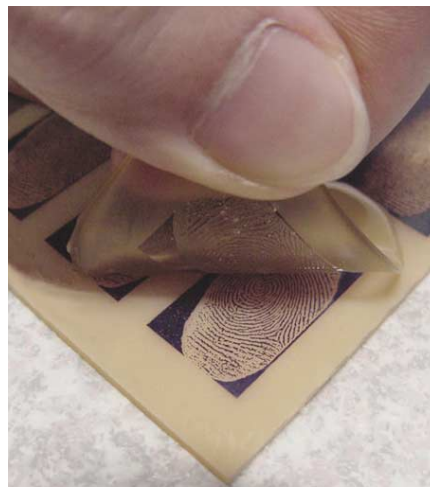
Keep 'em peeled: fake fingerprints can readily be made using gelatin and a simple mould.
