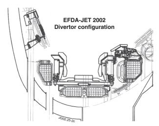
studies started in campaigns C1-C4 will be further extended this year in all three regimes. The removal of the septum in the divertor (fig. left) will allow an assessment of its contribution in establishing the excellent results of the 2000-2001 campaigns. The final aim is to obtain an integrated operational scenario combining the necessary conditions for use on ITER: high confinement, high density and an acceptable power and particle exhaust.
